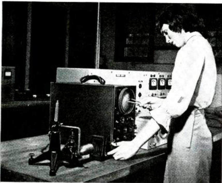
Operator sets dividers to exact width of pulse as she clicks camera shutter.
